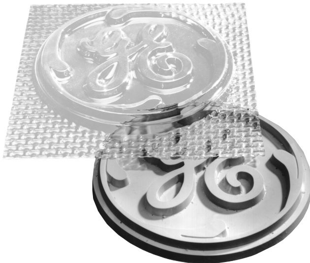
Fig. 1.14: Typical Vacuum Forming Mould
